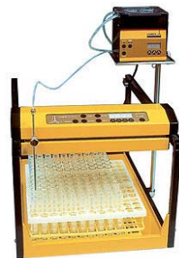
Automated fraction collector and sampler for chromatographic techniques
